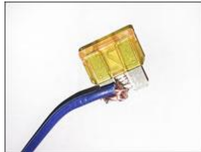
Wire Jammed Into a Fuse
