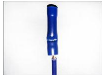
Broken Butt Connectors
