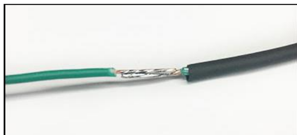
Soldered Connection w/ adhesive heat shrink
