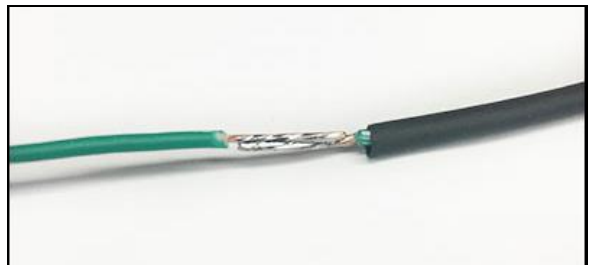
Soldered Connection w/ adhesive heat shrink
