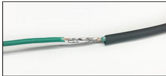
Soldered Connection w/ adhesive heat shrink
