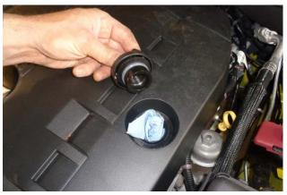
4. Remove the oil fill cap and temporarily protect the open fill neck with a clean paper towel.
