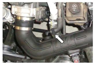
24. Install pinch clamp (24) on PCV hose, then install hose on elbow, checking for secure installation.
