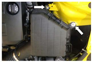
9. Remove the 2 airbox nuts. Firmly lift the airbox straight up to release it from its rubber grommet, then carefully remove the airbox and intake tube from the vehicle. **Retain nuts for reinstallation at Step 16.**
