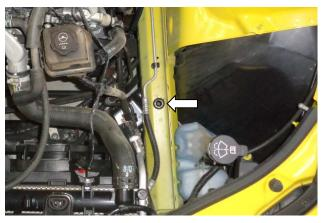
15. Place rubber well nut (18) in the mount hole that the grommet was removed from in Step 10.
