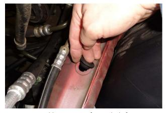
10. Remove rubber grommet from vehicle frame.
