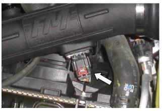
25. Reinstall the connector on the MAF sensor and close the locking tab, checking that the connector is secure.
