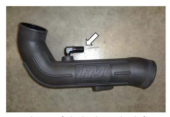
17. Apply 2 wraps of nylon thread tape to threads of PCV elbow (25), and install elbow into intake tube (23).
