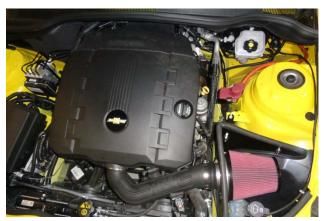
26. Remove the oil fill cap and temporarily protect the open fill neck with a clean paper towel. Reinstall the engine heat shield, remove the paper towel from the fill neck, and reinstall the fill cap.
