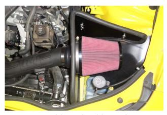
23. Install clamp (2) on air filter (1), install filter on filter adapter and tighten clamp.
