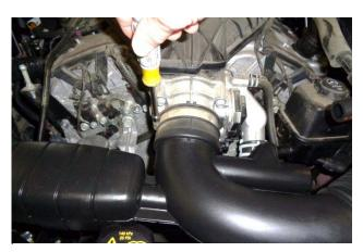
8. Loosen the hose clamp that secures the intake tube to the throttle body.
