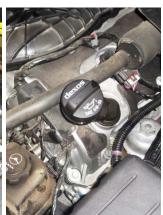
Remove the engine heat shield, then remove the paper towel from the fill neck and reinstall the fill cap.
