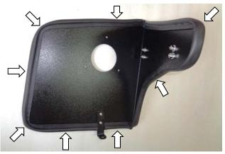
13. Attach rubber trim seal (9) to airbox. Starting next to bracket (17), press trim seal fully onto edge of airbox, slowly working around the airbox. When you return to the other side of bracket (17), trim the seal to fit using metal cutting shears.
