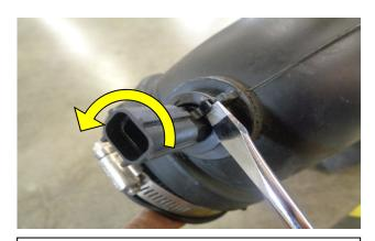
5. Remove the air temperature sensor from the factory intake tube by prying the clocking tab outward with a flat screwdriver and rotating counterclockwise as shown.
