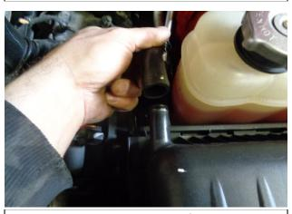
2. Disconnect crank case vent hose from stock air-box.
