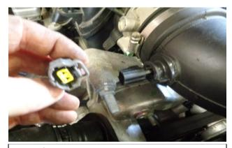
1. Carefully remove air temp. sensor connection.
