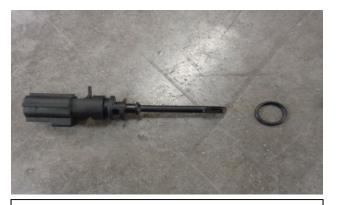
6. Remove the o-ring from the stock air temperature sensor and lubricate the o-ring area with a small amount of sensor-safe silicone grease or equivalent lubricant. Retain sensor for reinstallation later.
