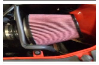
16. Secure the provided cone filter using the included hose clamp in the desired position. Recheck torque on all fasteners and clamps, reinstall the engine cover and reattach the negative battery cable.
