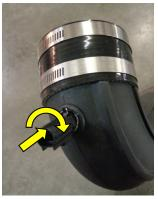
13.Install the included rubber grommet into the hole on the FM intake tube elbow and insert the air temperature sensor to the fully-seated position as shown by twisting clockwise and pressing inward .
