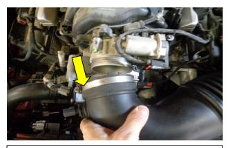
3. Loosen the hose clamp which secures the factory intake tube to the throttle body. Pull the tube away from throttle body and let it hang in place.
