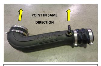
12. Carefully thread the included 90 degree barbed fitting into the brass threaded insert on the intake tube. Do not exceed 8 ft/lbs torque; if necessary, apply Teflon thread tape to achieve proper clocking and torque.
