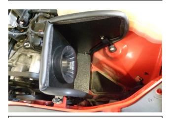
10. Install the heat shield assembly (minus the intake tube and air filter) into the vehicle as shown above with the well-nut expanded tight into the hole on the fender. Reinstall front cross frame bolt and tighten.
