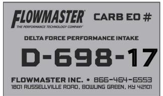
17. Affix the CARB EO label (25) to a clean, readily-visible location under the hood (e.g., near the hood latch).
