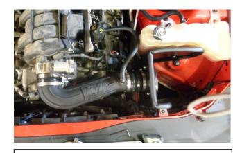
14. Install the FM intake tube assembly onto the airbox and the throttle body. Align and tighten all hose clamps for a satisfactory fit. Attach crankcase vent hose, pinch clamp, and air temperature sensor plug \* (see below).
