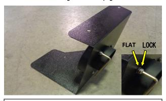
7. Begin by installing the filter adapter onto the heat shield as shown. Fasten with three 6mm screws with flat and locking washers in the sequence shown. Tighten securely but avoid over-torque.
