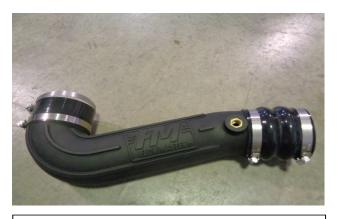
11. Loosely assemble the provided silicone-rubber couplers and corresponding hose clamps onto the FM intake tube as shown.
