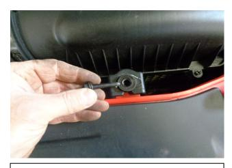
4. Remove the bolt for the factory air-box on the radiator core support and retain for later use. Remove the entire factory air-box/intake tube assembly by lifting straight up and out. NOTE: We highly recommend that customers retain their factory air intake system.
