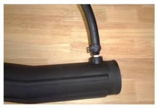
19. Install 5/8" ID hose (25) on the barbed fitting and secure with pinch clamp (26). (Install full length of hose; it will be cut to length later.)
