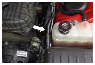
5. Carefully pull the hard plastic breather line from the hose on the airbox.
