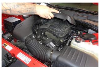
4. Remove the engine cover by firmly lifting at each corner to release it from its four friction clips.
