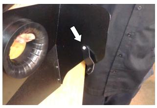
13. Attach bracket (4) to heat shield using ¼-20 screw(5) (against the bracket), and nut (7), lock washer(8) and flat washer (9) (against the heat shield). Do not fully tighten hardware at this time.
