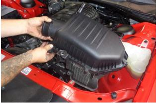
9. Remove the airbox from the vehicle.
