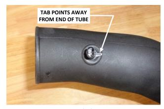
18. Install rubber grommet (18) in intake tube.
