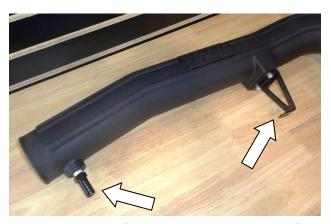
17. Apply 2 wraps of nylon thread tape to threads of 5/8" fitting (27), and install it in the intake tube (15). Attach bracket (16) to intake tube using M6 screws (12), lock washers (11), and flat washers (10). Do not tighten bracket hardware at this time.
