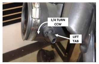
10. Remove the air temp sensor from the intake duct by lifting the locking tab, then turning the sensor a quarter-turn counter-clockwise. Then remove the o-ring from the sensor. **CAUTION: The sensor is delicate!** Handle it with care, and store it in a safe location until reinstallation.
