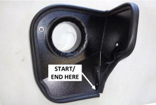
14. Attach gasket (30) to heat shield. Starting at the corner shown, firmly press the gasket onto the edge, gradually working around the heat shield. When you return to the starting point, trim the gasket to fit using metal-cutting shears.
