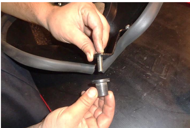
14. At bracket (5), thread the well nut (4) onto the ⅜-16 screw (6). NOTE: Hand tighten only at this time.
