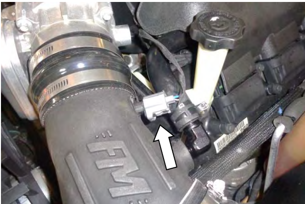
19. Reinstall connector on the intake air temperature sensor and verify that the connector is secure.
