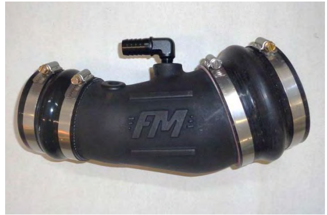
15. Install two small hose clamps (16) on small flex coupler (15), and install coupler on throttle body side of intake tube. Install two large hose clamps (20) on large flex coupler (13), and install coupler on air filter side.
