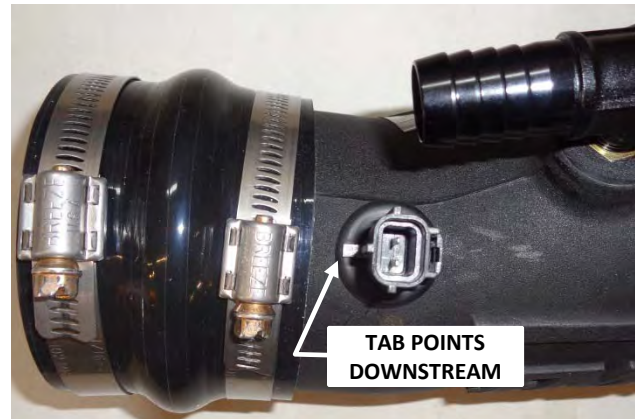
16. Carefully insert the intake air temperature sensor into the grommet, ensuring that the tab points downstream. (NOTE: Moistening the grommet with soapy water will ease insertion.)
