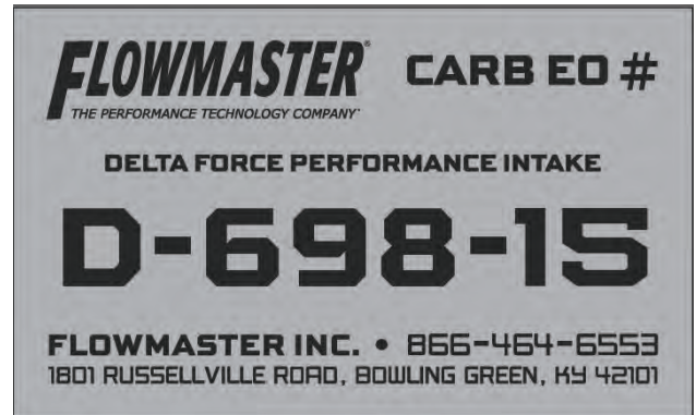
21. Affix the CARB EO label (25) to a clean, readily-visible location under the hood (e.g., near the hood latch).
