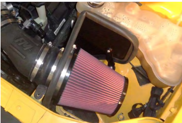
20. Install clamp (2) on air filter (1), install filter on filter adapter and tighten clamp.
