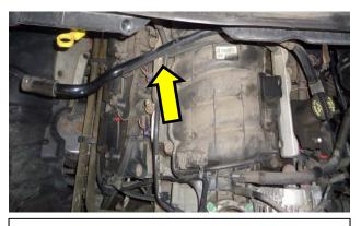
7. Remove the crankcase vent tube prom the engine. Replace the stock tube with the included hose/clamps. Route in the same path, trimming off any excess length after install of the FM system.
