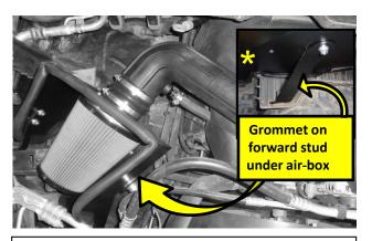
15. Insert the assembled FM intake system into the vehicle as shown\*. Attach the extended crankcase vent hose/clamp. Connect the air temperature sensor plug and secure the intake tube on the throttle body.
