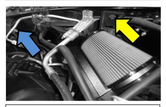
16. Reinstall the two previously removed bolts on the fender → and the front cross-frame → to secure the FM air-intake assembly. Check all fitment /fasteners and reattach the negative battery cable.
