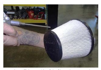
2. <u>Blow off the outside</u> of the filter. Blow across the filter surface (at about a 45° angle), not through the filter material. Hold the air nozzle about 6 inches away from the filter surface, always keep it moving, and point the air jet in to—not across—the pleats.
