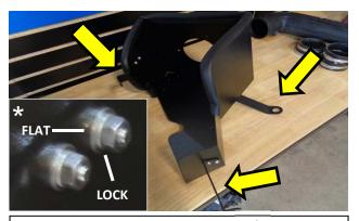
10. First, attach the 3 metal brackets 🖵 to the FM heat-shield using the supplied ¼" bolts/nuts and corresponding flat/lock washers installed under the nut-side as shown\*. Tighten all fasteners securely.
