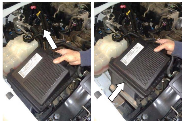
11. To remove the stock airbox, grasp the inlet side and lift it straight up to release the 2 mount pins from their rubber grommets. Then slide the airbox inboard to release it from the airbox shelf.
