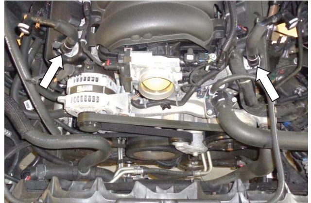
10. Remove both PCV hoses from the valve covers by depressing their release latches and pulling straight off.
