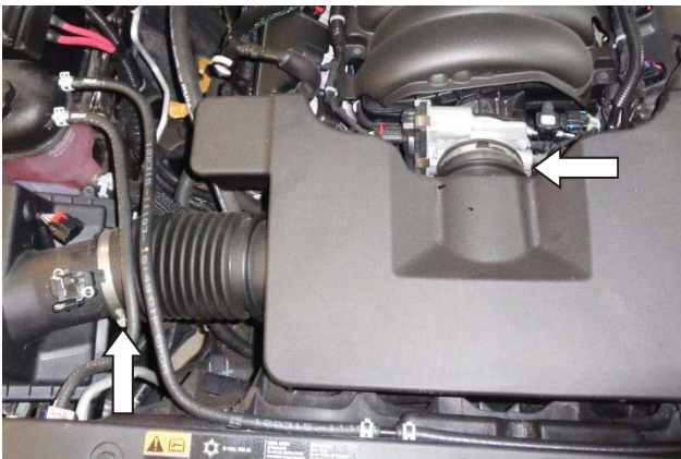
8. Loosen the two screw clamps shown – one at the airbox, and the other at the throttle body.
