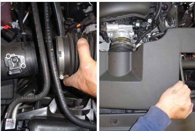
9. Separate the intake duct from the airbox, separate the intake plenum from the throttle body, and carefully remove the assembled duct and plenum from the vehicle.
