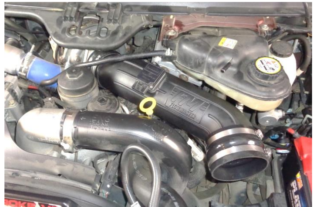
24. Push the coupler onto the turbo inlet.
