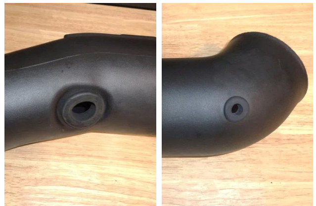
18. Insert the rubber grommets (22) and (19) in their holes in the intake tube (18). Moistening the grommets with soapy water will ease insertion.
