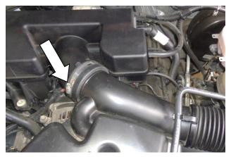
11. Loosen the screw clamp between the intake duct and resonator and remove the duct from the vehicle.
