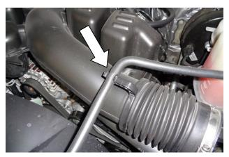
7. Release the coolant hose from the clip on top of the intake duct.
