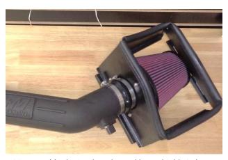
22. Assemble the intake tube and heat shield. Only snug – do not tighten – the tube clamp at this time.
