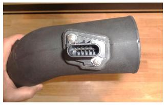
21. Install the MAF sensor gasket (11) over the sensor, then install the sensor in the intake tube, ensuring the correct orientation of the gasket and sensor to the mount pad. Secure the sensor using M4 screws (12).
