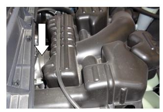
10. At the back of the resonator, loosen the screw clamp between the resonator and the throttle body.
