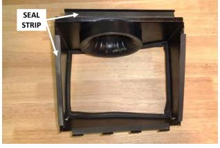
17. Cut the adhesive seal strip (19) to the lengths required, and apply it to the four bottom edges of the heat shield.
