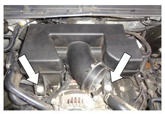
12. Remove the two bolts at the front of the resonator, then disconnect the resonator from the throttle body and remove it from the vehicle.
