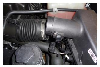
Separate the intake duct from the airbox cover.
