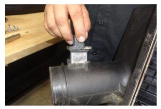
Remove the MAF sensor from the airbox cover, then remove the factory gasket from the sensor.
