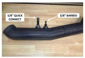
20. Your vehicle may require either the 5/8" quick connect fitting (15), or the 3/8" barbed fitting (13), or both. If it uses only one fitting, install the 1/4" plug (20) in the unused port. Apply 2 wraps of nylon thread tape to threads of the required hardware, and install them in the intake tube (10).
