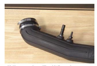
23. Place screw clamps (8) and (16) onto the coupler (17). Install the coupler on the other end of the intake tube. Only snug – do not tighten – the tube clamp at this time. (Leave the other clamp loose.)
