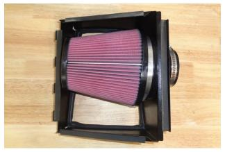
19. Slip screw clamp (2) onto air filter (1), then install the filter on the filter adapter and tighten the clamp.
