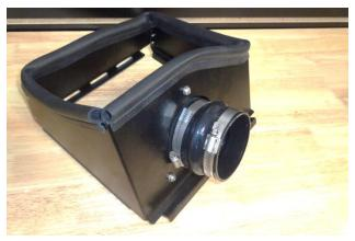
18. Place (x2) screw clamps (8) onto the 3-1/2" coupler (9). Install the coupler on the air filter adapter, pushing it flush against the heat shield. Tighten only the filter adapter clamp at this time. (Leave the other clamp loose.)
