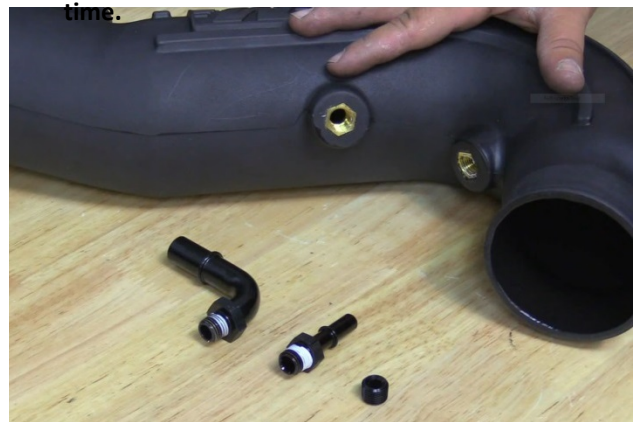
24. Determine which vacuum fitting(s) are needed for your vehicle's configuration. The 5/8" elbow (18) mates with the PCV hose. The 3/8" straight (19) mates with the EVAP hose. The 1/4" plug (20) will be installed if only one vacuum fitting is used.
