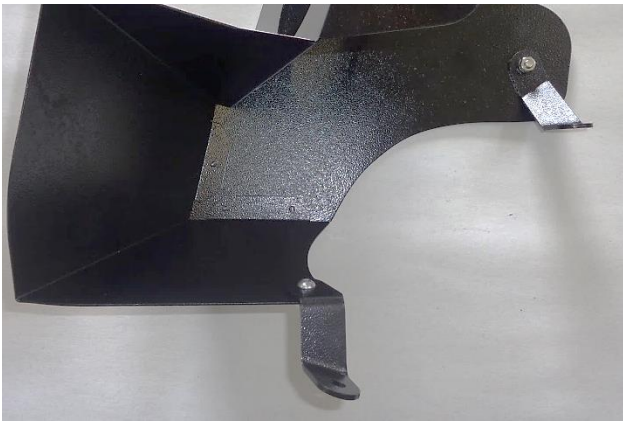
20. Attach bracket (10) to heat shield using ¼-20 × 5/8" screw (21) (against the bracket), and flat washer (22), lock washer (23) and nut (24) (against the heat shield). Do not tighten the fasteners at this time.
