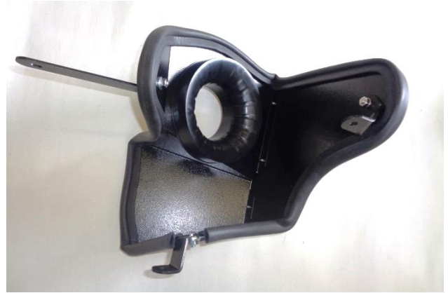
22. Attach the gasket (25) to the heat shield. Starting on one side of bracket (10), gradually work around the heat shield, firmly pressing the seal onto the edge. When you return to the bracket, trim the gasket to fit using metal-cutting shears.
