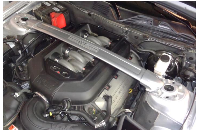
35. Reinstall the engine appearance cover. If applicable, reinstall the strut tower brace, tightening the strut tower nuts to the torque value specified by the vehicle manufacturer.
