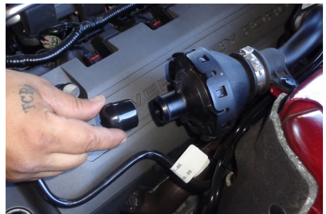
17. Push the vinyl cap (11) onto the resonator.
