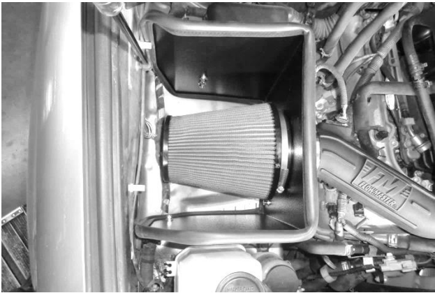
37. Install clamp (2) on air filter (1), install filter on filter adapter and tighten clamp.
