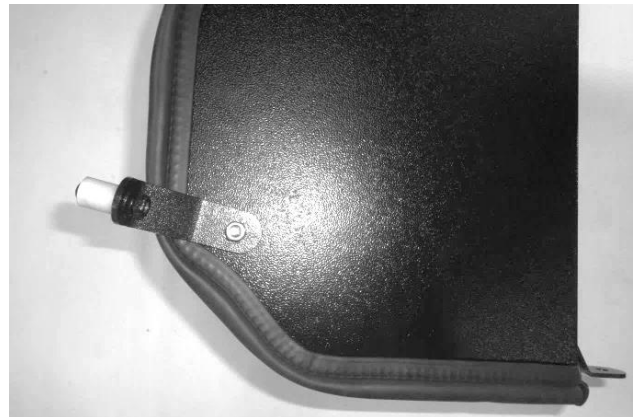
22. Attach bracket (26) to airbox using \frac{1}{4} -20 \times 5/8" screw (28) and flat washer (25) (against airbox), and nut (7) and lock washer (8) (against bracket). Leave bracket slightly loose until installation of airbox.
