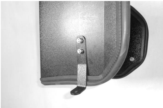
19. Attach bracket (3) to airbox using \frac{1}{4} -20 \times 5/8" screws (28) and flat washers (25) (against airbox), and nuts (7) and lock washers (8) (against bracket).
