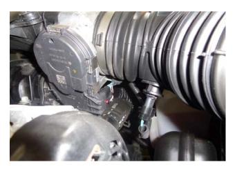
3. Disconnect the electrical plug from the air temperature sensor located on the underside of the intake tube near the throttle body by depressing the backside of the rocking tab and gently pulling away.
