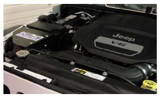
17. Secure the provided cone filter using the included hose clamp in the desired position. Using the last three  $\frac{1}{2}$ " screws/washers, secure the air-box lid, reinstall the engine cover and the battery cable.
