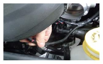
16. \*Due to limited space for access, it may be necessary to attach the air temperature plug during the intake tube attachment process. Make sure that the plug fully engages the retaining tab on the sensor.
