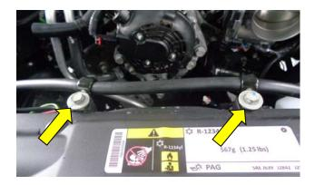
14. Use the retained stock front cross-frame air tube/resonator bolts and the provided vinyl coated loom-clamps to secure the coolant overflow tube to the cross-frame. Do not over-tighten.
