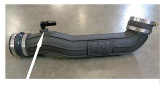
\*Do not exceed 8 ft/lbs torque; if necessary, apply Teflon thread tape to achieve proper clocking/torque.
