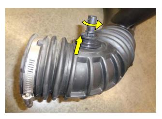
5. Remove the entire stock intake assembly from the vehicle by lifting straight up and out. Turn upsidedown on a flat surface and remove the air temp sensor from the intake tube by prying up the clocking tab with a flat screwdriver and rotating c-clockwise.
