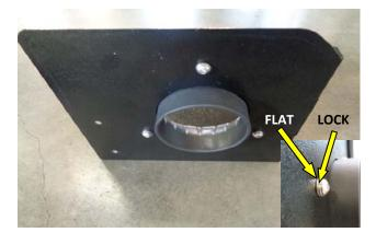
8. Begin by installing the air-filter adapter onto the heat shield as shown. Fasten with three 6mm screws placing the flat and locking washers in the sequence shown. Tighten securely but avoid over-torque.
