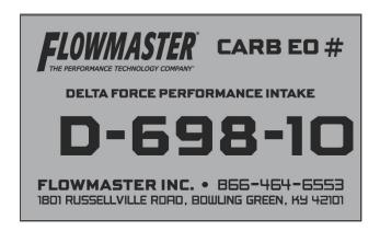
18. Affix the CARB Exemption Order label to a clean, readily-visible location under the hood (e.g., near the hood latch), so an inspector can easily see it at emissions testing.
