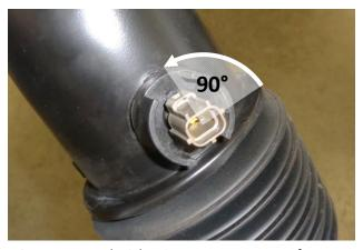
8. To remove the inlet air temperature sensor from the intake duct, lift the locking tab, rotate it a quarter-turn counter-clockwise, then pull. Remove the o-ring from the sensor. **CAUTION: The sensor is delicate!** Handle it with care, and store it in a safe location until reinstallation.
