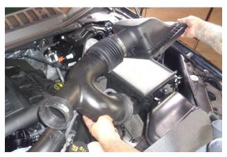
Remove the assembled intake duct and airbox cover from the vehicle, then remove the stock air filter.
