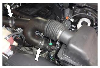
4. Loosen (x2) screw clamps on air intake duct as indicated.
