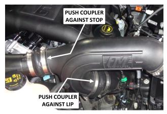
18. Push each coupler up against its stop on the turbo duct and tighten its turbo duct clamp. Then "center" the intake tube between the couplers (so that there are approximately equal amounts of tube inserted in each coupler), and tighten the three screw clamps on the intake tube.
