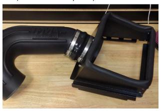
13. Assemble the intake tube (13) and heat shield, then partially tighten clamps.
