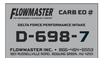
20. Affix the CARB Exemption Order label to a clean, readily-visible location under the hood (e.g., near the hood latch), so an inspector can easily see it at emissions testing.
