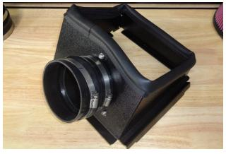
12. Slip 2 of the large screw clamps (11) onto the 4-1/2" coupler (10). Install the coupler onto the air filter adapter, pushing it flush against the heat shield. Tighten only the filter adapter clamp at this time. (Leave the other clamp loose.)
