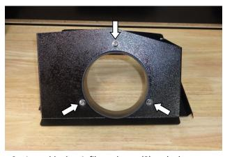
9. Assemble the air filter adapter (3) to the heat shield (5) using the M6 screws (9), lock washers (8) and flat washers (7).
