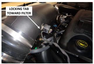
19. Carefully push the inlet air temperature sensor into the grommet and point the locking tab toward the air filter. (Moistening the hole with soapy water will ease insertion.) Reinstall the sensor plug and verify that the connection is secure.
