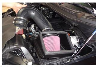
16. Insert the four tabs on the heat shield into the slots on the back of the airbox. Lower the intake tube and slip the two couplers over their turbo ducts. Do not tighten the clamps at this time.
