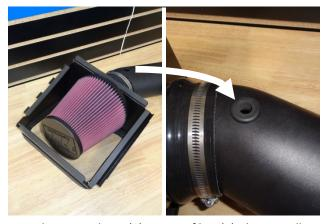
15. Slip screw clamp (2) onto air filter (1), then install the filter on the filter adapter and tighten the clamp. Install grommet (12) in intake tube. (Moistening the hole with soapy water will ease insertion.)
