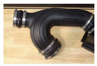
14. Slip (x2) screw clamps (11) onto 4-1/2"-4" coupler (14) and (x2) screw clamps (16) onto 3-1/2" -4" coupler (15). Place both couplers onto intake tube then partially tighten each screw clamp.
