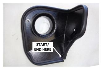
12. Attach gasket (24) to heat shield. Starting at the corner shown, firmly press the gasket onto the edge, gradually working around the heat shield. When you return to the starting point, trim the gasket to fit using metal-cutting shears.
