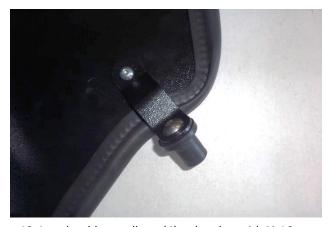
13. Attach rubber well nut (4) to bracket with %-16 screw (11), hand tight only.
