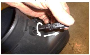
8. Remove the temp sensor from the airbox by gently lifting the locking tab outward with a flat screwdriver and rotating the sensor counter-clockwise. Remove o-ring from temp sensor and retain sensor for re-use.
