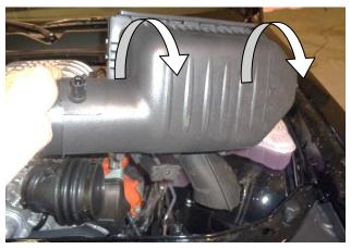
Remove the airbox by simultaneously lifting it up and rolling it forward. Then, remove the air duct from the throttle body.
