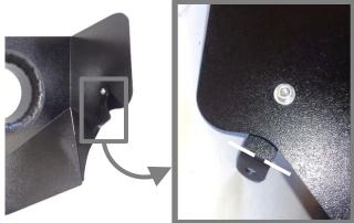
11. Attach bracket (5) to heat shield using ¼-20 screw (9) (against the bracket), and flat washer (6), lock washer (7) and nut (8) (against the heat shield).
