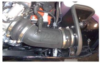
17. Install the intake tube in the vehicle. Carefully press the crankcase vent hose into the large grommet. (NOTE: Moistening the grommet with soapy water will ease insertion.) Then reconnect the air temp sensor plug.
