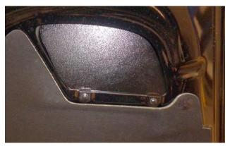
20. Install the block-off plate using the two stock screws. **CAUTION: Use only the stock screws, to avoid damaging the hood.**
