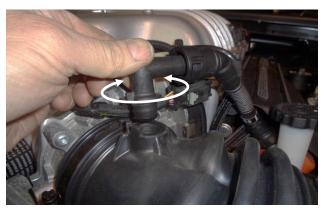
Disconnect the crankcase vent hose from the air duct by pulling straight up while also rocking it around in an orbital motion. Spraying a rubber-safe lubricant around the opening will ease removal.
