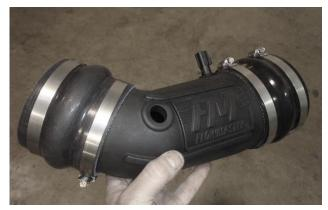
16. Install two small hose clamps (21) on small flex coupler (22), and install coupler on discharge end of intake tube. Install two large hose clamps (16) on large flex coupler (17), and install coupler on intake end of tube.
