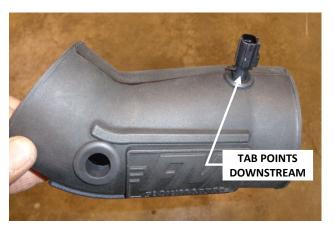
15. Insert rubber grommets (19) and (20) in the intake tube (18). Carefully press the air temp sensor into the small grommet, ensuring that the tab points downstream. (NOTE: Moistening the grommet with soapy water will ease insertion.)
