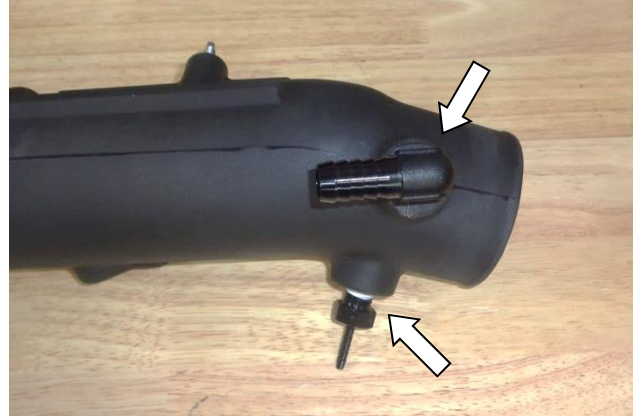
22. Apply 2 wraps of nylon thread tape to the 5/8" elbow (27) and the 3/16" straight fitting (31), and install them in the intake tube, orienting the elbow as shown.
