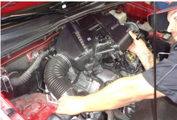
14. Carefully remove the assembled intake duct and airbox from the vehicle.
