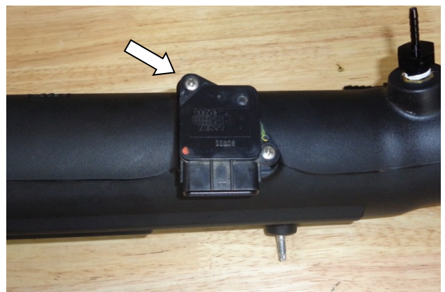
24. Install MAF sensor gasket (28) on the sensor and adaptor, then install the sensor in the intake tube using M4 screws (30).
