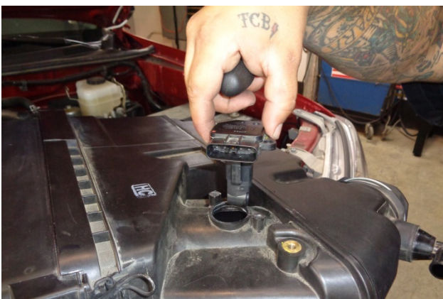
15. Remove the mass airflow (MAF) sensor from the airbox. Do not remove the o-ring from the sensor.
