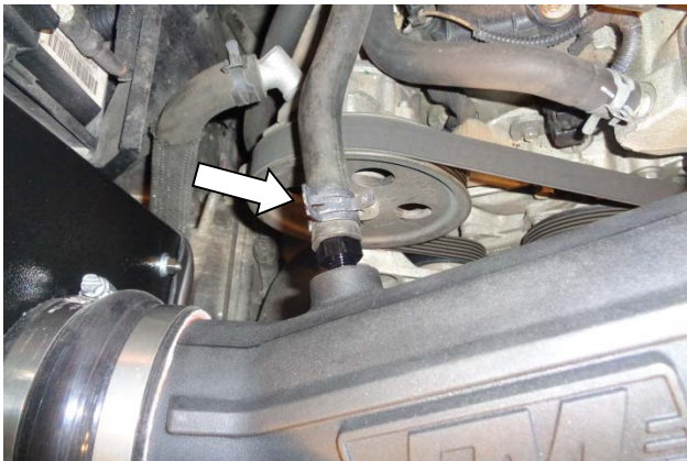
20. Secure PCV hose on barbed fitting with pinch clamp (17).
