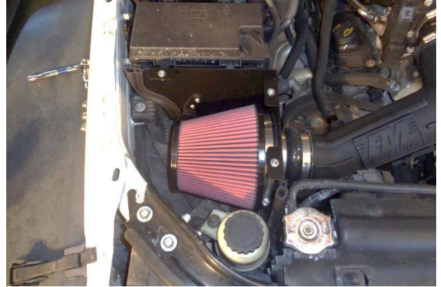
22. Install clamp (2) on air filter (1), install filter on filter adapter and tighten clamp.
