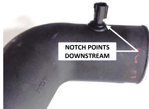
16. Carefully insert the intake air temperature sensor into the grommet, ensuring that the notch in its base points downstream. NOTE: Moistening the grommet with soapy water will ease insertion.
