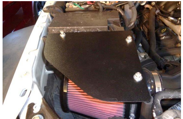
23. Install airbox cover (7) on airbox, using ¼-20 screws (10), lock washers (9), and flat washers (8).
