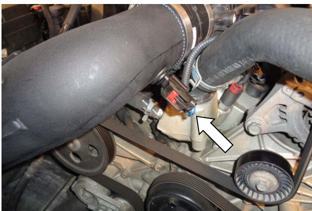
21. Reinstall the intake air temperature sensor connector and verify the connector is secure.
