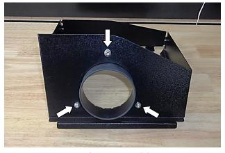
Assemble the air filter adapter (3) to the heat shield (4) using the M6 screws (9), lock washers (8) and flat washers (7).
