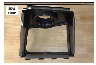
11. Cut the adhesive seal strip (5) to the lengths required, and apply it to the four flat edges of the heat shield.
