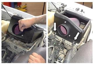
13. Insert the four tabs on the heat shield into the slots on the side of the stock airbox. Secure the heat shield to the airbox with the front and rear latches only. NOTE: The center latch will not be used, and may be removed if desired.
