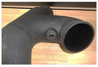
15. Apply 2 wraps of nylon thread tape to the threads of the plug (13), and install it in the intake tube.
