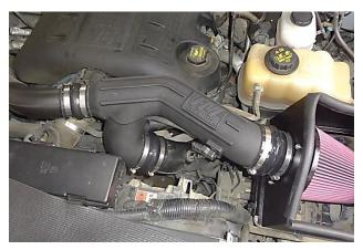
18. Install the intake tube in the vehicle, slipping the couplers over the two turbo inlets and filter adapter.
