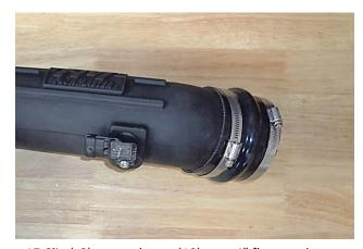
17. Slip (x2) screw clamps (10) onto 4" flex coupler (11). Push coupler onto intake tube then partially tighten tube clamps.
