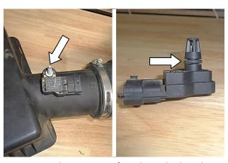
8. Remove the MAF sensor from the intake duct, then remove the o-ring from the sensor. **CAUTION: The sensor is delicate!** Handle it with care, and store it in a safe location until reinstallation.
