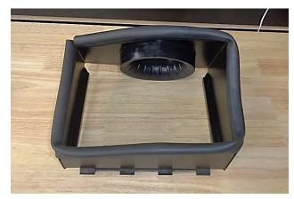
10. Attach the gasket (6) to the heat shield. Firmly press the gasket onto the heat shield, gradually working your way around. When you return to the starting point, use metal-cutting shears to trim the gasket to length.
