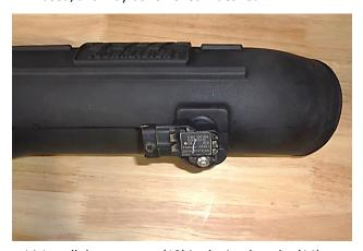
14. Install the grommet (12) in the intake tube (14). Then install the sensor in the grommet using the M6 screw (9). (Soapy water will ease insertion of the grommet in the tube, and the sensor in the grommet.)
