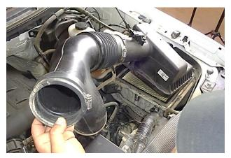
7. Separate intake duct from (x2) turbocharger inlets then remove intake duct and airbox cover as a unit. Remove the stock air filter.
