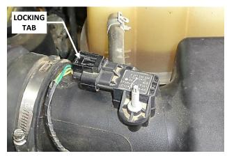
5. Disconnect the electrical plug from the Mass Airflow (MAF) sensor by squeezing the locking tab, then pulling the plug straight off the sensor.
