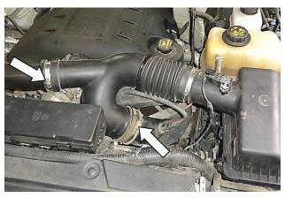
4. Loosen (x2) screw clamps on air intake duct.
