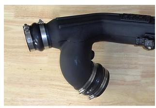
16. Slip (x2) screw clamps (16) onto 3" flex coupler (15). Slip (x2) screw clamps onto 4" flex coupler (11). Push each coupler onto intake tube then partially tighten tube clamps.
