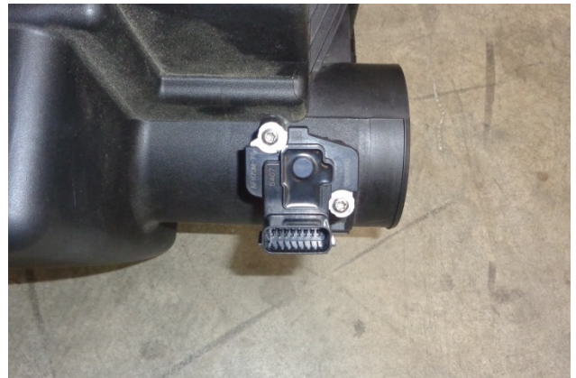
12. Remove the MAF sensor from the airbox, then remove the factory gasket from the sensor. CAUTION: The sensor is delicate! Handle it with care, and store it in a safe location until reinstallation.
