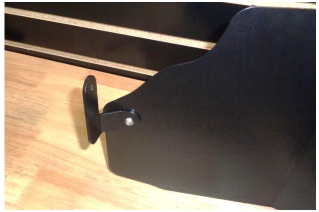
16. Attach bracket (7) to the heat shield using a 1/4-20 screw (8) (on the heat shield side), and a flat washer (6), lock washer (5) and nut (4) (on the bracket side). Do not fully tighten the fasteners at this time.
