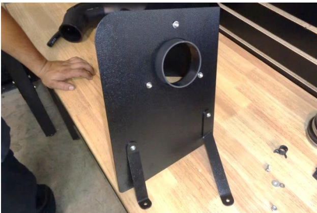
15. Attach brackets (12) and (15) to the heat shield using 1/4-20 screws (8) (on the bracket side), and flat washers (6), lock washers (5) and nuts (4) (on the heat shield side). Do not tighten the fasteners at this time.
