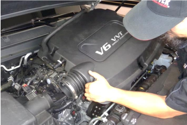
7. The engine cover and intake duct are one piece. Separate the intake duct from the airbox, then remove the cover and duct from the vehicle.
