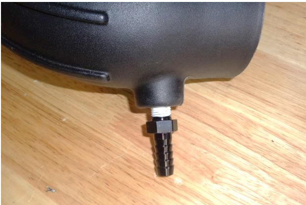
20. Apply 2 wraps of nylon thread tape to the 1/2" barbed fitting (23), and install it in the intake tube.
