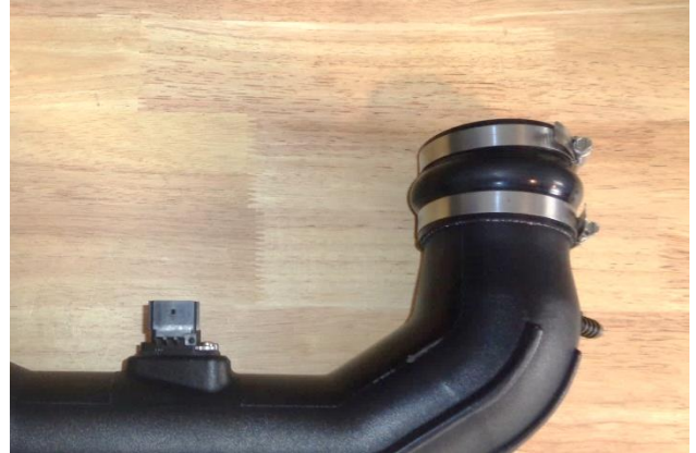
22. Install the two smaller screw clamps (20) on the 3" coupler (21), and install the coupler on the throttle-end of the intake tube. Do not tighten the clamps at this time.
