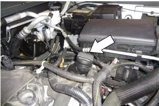
8. Reinstall the oil filler cap.
