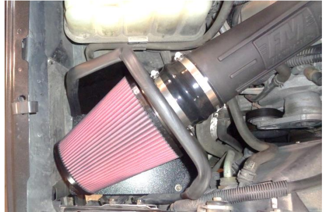
22. Slip screw clamp (2) onto air filter (1), install the filter on the filter adapter, and tighten the clamp.
