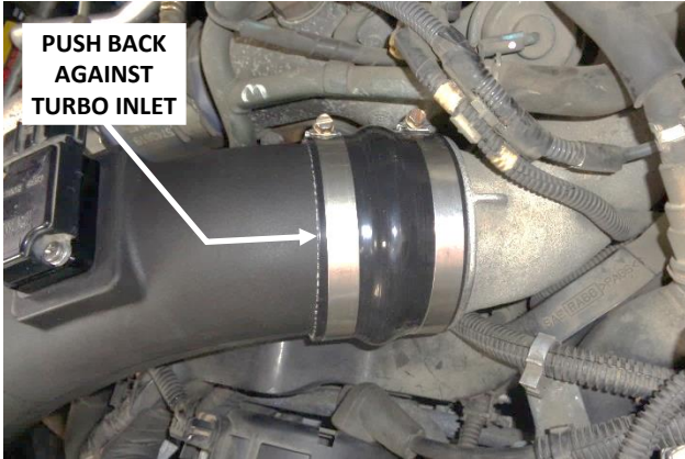
19. Push the small coupler back against the lip on the turbo inlet, and tighten only the turbo inlet clamp.
