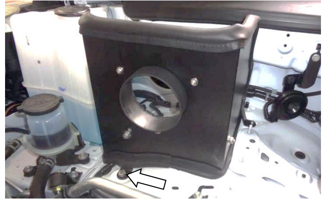
16. Fasten bracket (8) to the vehicle using the M8 bolt (14) and lock washer (13). After all 3 heat shield brackets are secured to the vehicle, tighten each bracket's fasteners to the heat shield.
