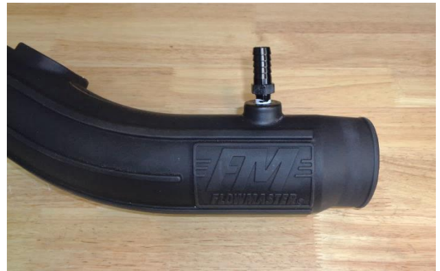
17. Apply 2 wraps of nylon thread tape to the 5/8" barbed fitting (24) and install it in the intake tube (20).
