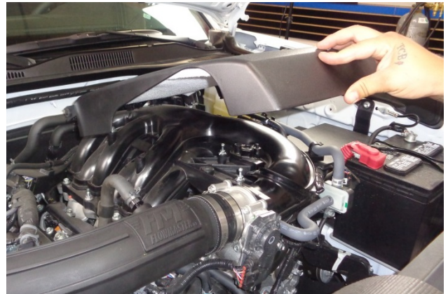
29. Reinstall the engine appearance cover.
