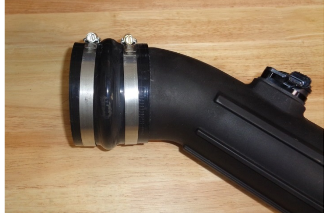
22. Install the two large screw clamps (18) on the large coupler (19), and install the coupler on the filter end of the intake tube. Do not tighten clamps at this time.
