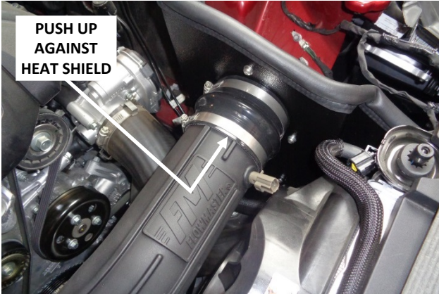
25. Push the large coupler flush up against the heat shield. Tighten only the clamp on the filter adapter.
