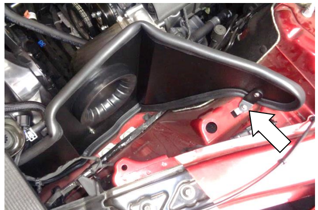
17. At the upper rear bracket, install and tighten the M6 screw (5), lock washer (6) and flat washer (7).
