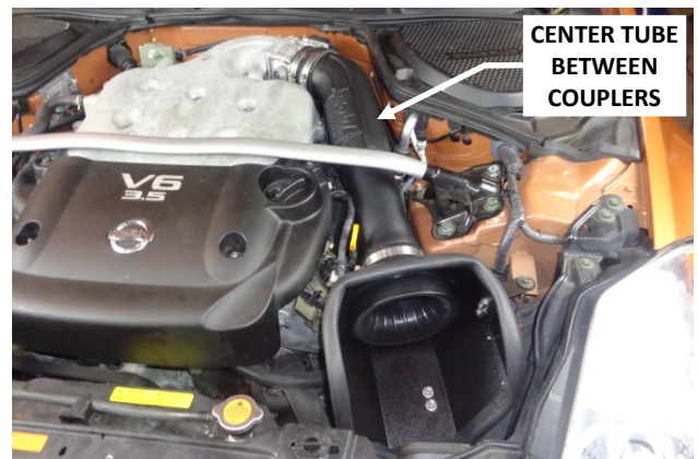
30. Center the intake tube between the couplers (so that roughly an equal amount of the tube is inside each coupler), and tighten the two remaining screw clamps.
