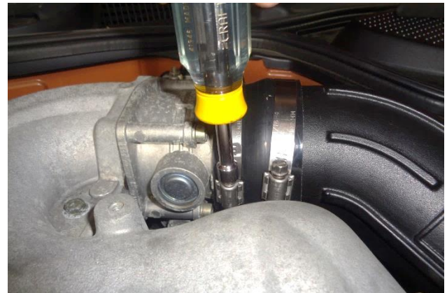
29. Tighten only the throttle body clamp.
