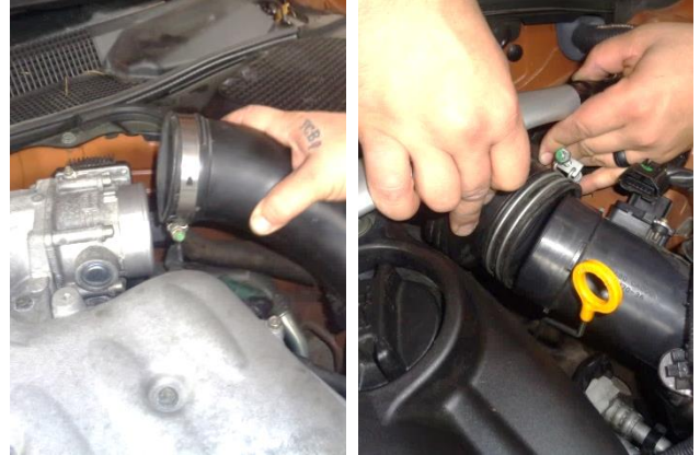
10. Separate the duct from the throttle body and the airbox, then carefully roll the duct slightly away from the engine.
