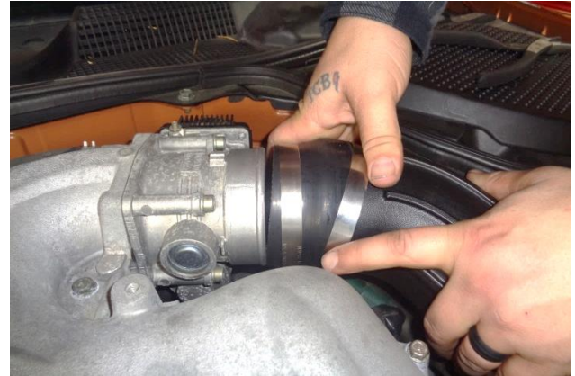
28. Push the coupler all the way onto the throttle body.
