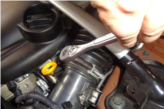
8. Loosen the screw clamp that secures the duct to the airbox.
