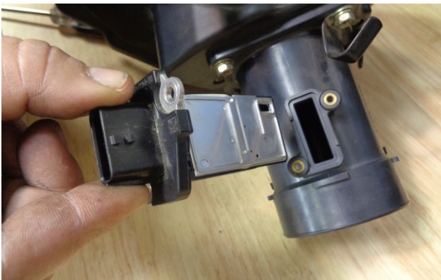
14. Remove the MAF sensor from the airbox, then remove the factory gasket from the sensor. CAUTION: The sensor is delicate! Handle it with care, and store it in a safe location until reinstallation.
