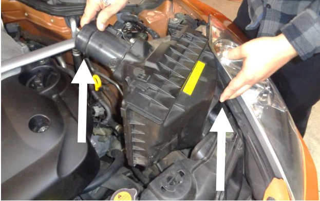
13. Remove the airbox from the vehicle by firmly pulling straight up.
