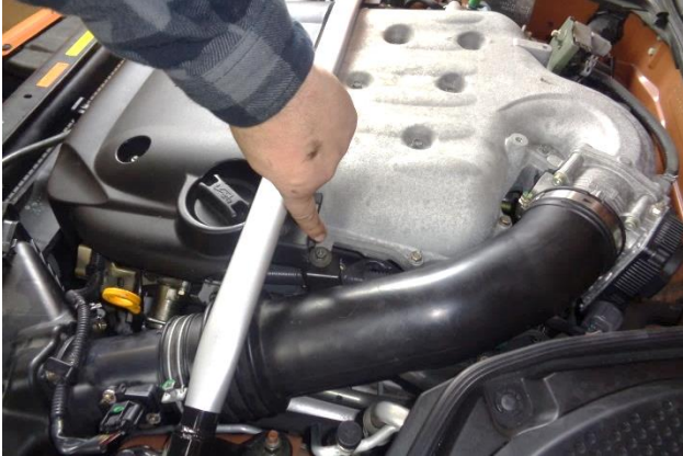
7. Remove the air duct bracket bolt.
