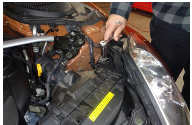
12. Remove the bolt that secures the airbox to the vehicle and retain it for use at Step 21 .
