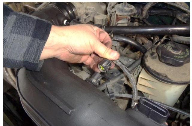
36. Connect the air temp sensor plug to the sensor and check the plug for security.
