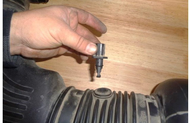
16. Firmly grasp and twist the air inlet temp sensor, and pull it from the inlet duct.
