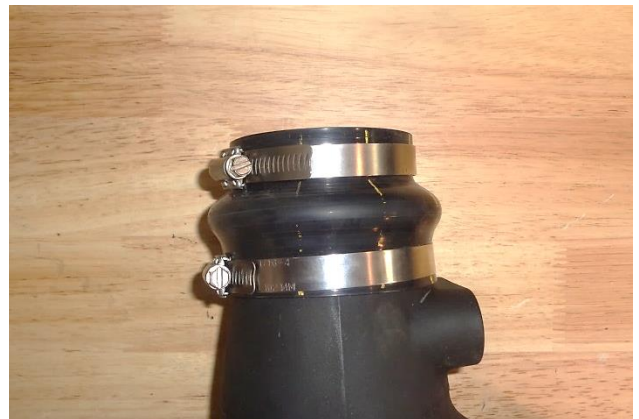
23. Install the medium screw clamp (24) and small screw clamp (26) on the 3-1/2" - to - 3" coupler (25). Then install the coupler on the throttle body end of the intake tube. Do not tighten the clamps at this time.
