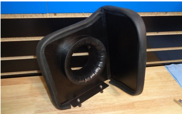
21. Attach the gasket (9) to the heat shield. Starting at one end, firmly press the gasket onto the edge of the heat shield, gradually working all the way around. When you return to the other end, trim the gasket to fit using metal-cutting shears.
