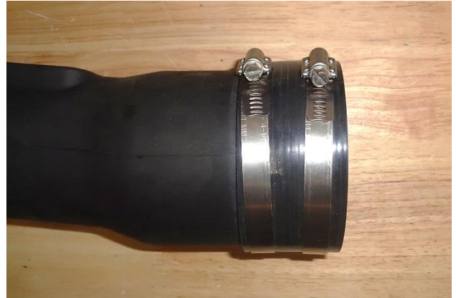
22. Install the 2 large screw clamps (10) on the 4" straight coupler (11). Then install the coupler on the filter end of the intake tube (21). Do not tighten the clamps at this time.
