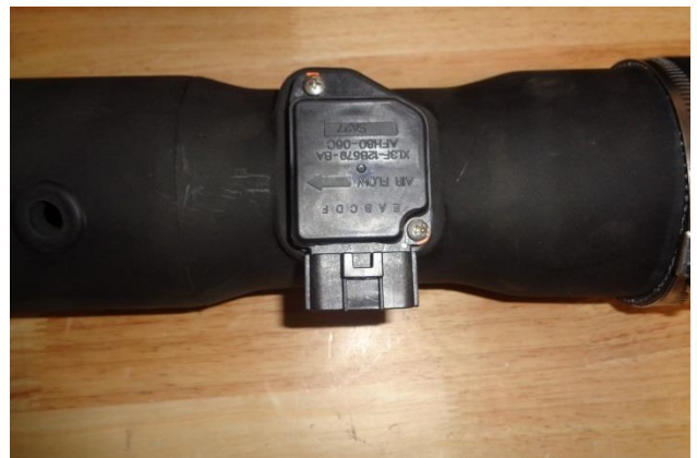
24. Install the MAF sensor gasket (12) onto the sensor, ensuring correct orientation. Then install the sensor in the intake tube, using the M4 screws (13).
