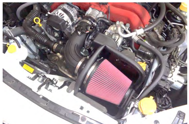
30. Slip screw clamp (2) onto air filter (1), install the filter on the filter adapter, and tighten the clamp.
