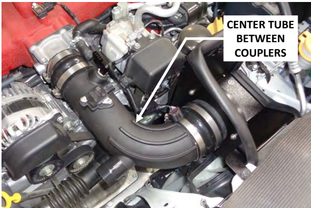
26. Center the intake tube between the couplers (so that there is roughly an equal length of tube inside each coupler), and tighten the two intake tube clamps.
