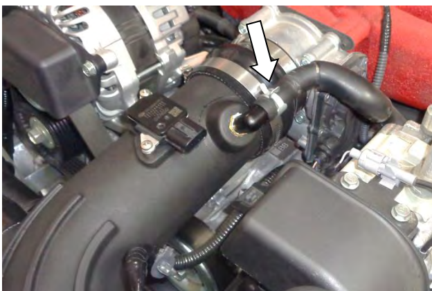
27. Align the barbed elbow with the breather tube, push the tube onto the elbow, and secure the tube with the pinch clamp.
