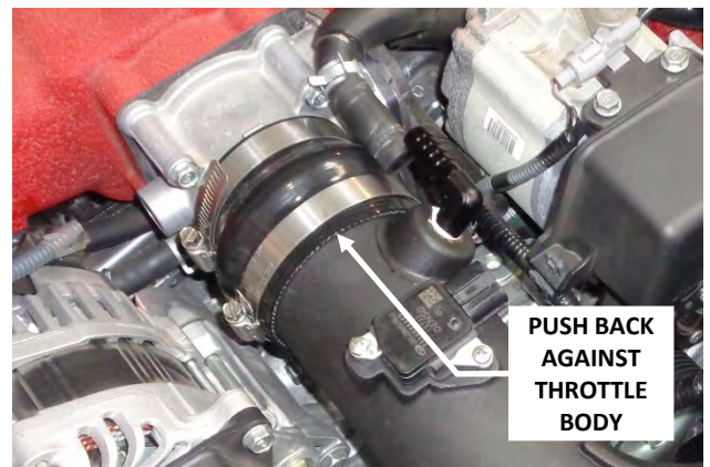
24. Push the rear coupler back against the stops on the throttle body, and tighten only the throttle body clamp.
