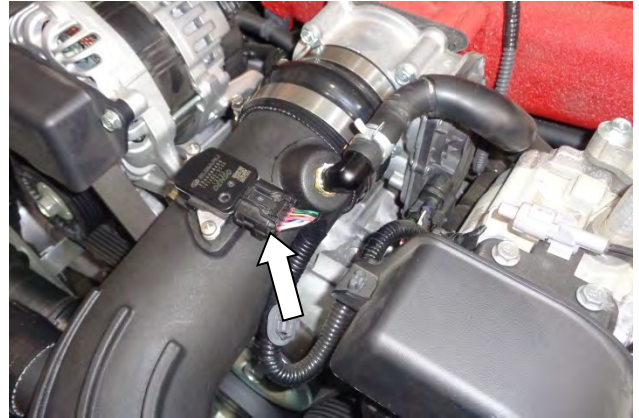
28. Push the MAF sensor plug onto the sensor until it clicks, then verify the connection is secure.
