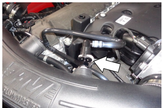
34. Connect the PCV line to the quick connect fitting, adjusting the PCV lines as necessary to align them. Verify that the connection is secure.
