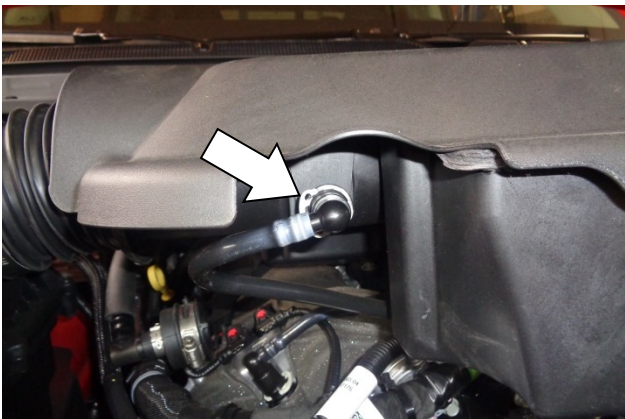
8. Carefully lift the engine cover and separate the intake duct from the throttle body. Then at the front of the cover, depress the latch and pull the PCV line straight off the intake duct.
