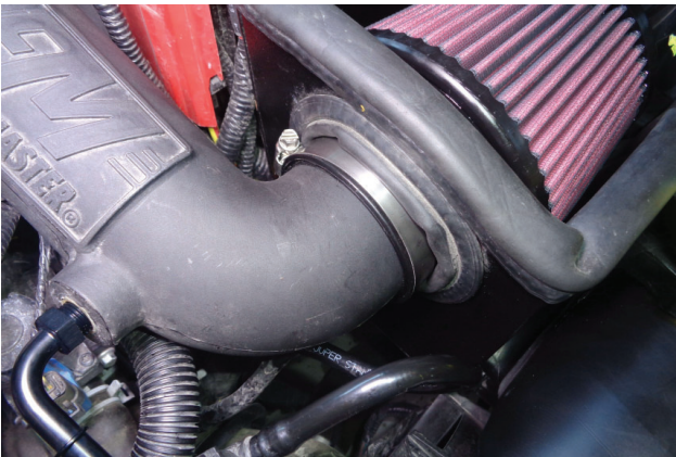
32. Ensure that there is a minimum ½" overlap between the intake tube and the filter flange, then tighten the screw clamp. NOTE: When tightened, a small margin of the clamp may sit under the gasket.
