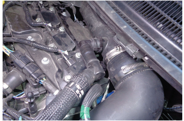
34. Reconnect the PCV tube to its port on the turbo inlet, then verify that the connection is secure.
