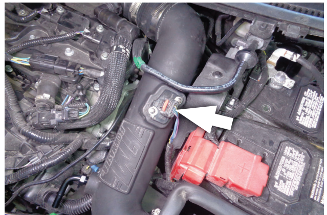
35. Connect the MAF sensor plug to the sensor, close the latch, and check the connection for security.
