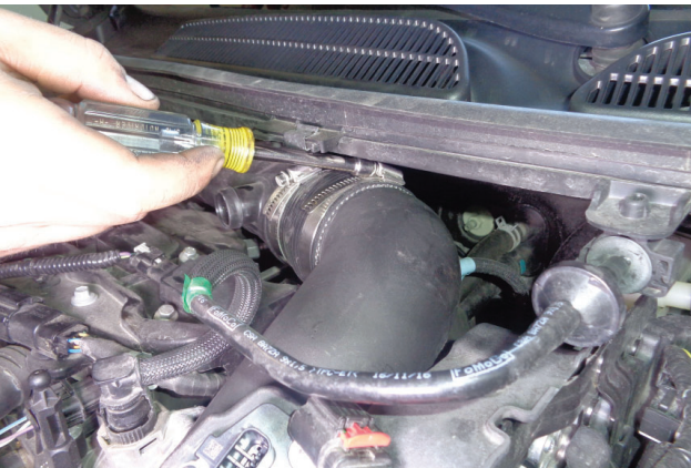
33. Tighten the coupler clamp at the intake tube.
