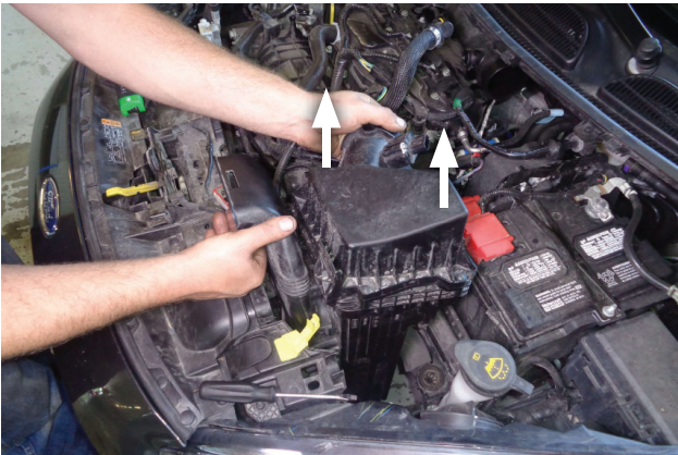
14. Remove the airbox and ram air duct from the vehicle.
