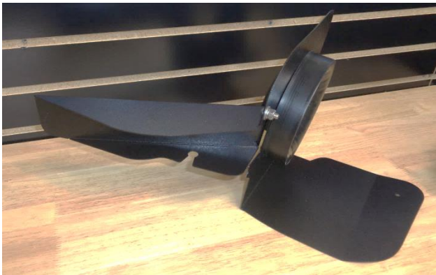
20. Assemble the inlet air duct (5) to the heat shield using a ¼-20 screw (9) (on the duct side), and a flat washer (8), lock washer (7) and nut (6) (on the heat shield side).
