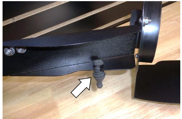
23. Push the rubber mount pin removed from the airbox at Step 17 into the notch in the inlet air duct as shown.
