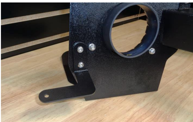
21. Attach bracket (16) to the heat shield using ¼-20 screws (9) (on the bracket side), and flat washers (8), lock washers (7) and nuts (6) (on the heat shield side).
