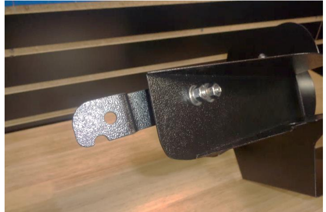
22. Attach bracket (10) to the inlet air duct using ¼-20 screws (9) (on the bracket side), and flat washers (8), lock washers (7) and nuts (6) (on the duct side).
