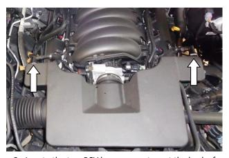
6. Locate the two PCV hose connectors at the back of the intake plenum as shown.
