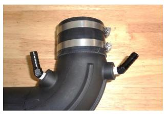
19. Slip 2 screw clamps (8) onto the small coupler (11). Push the coupler onto the throttle body-end of the intake tube. Snug the tube clamp (do not tighten at this time), and leave the other clamp loose.
