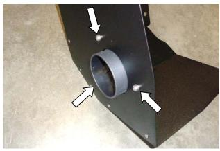
14. Assemble the air filter adapter (3) to the heat shield (4) using the M6 screws (7), lock washers (6) and flat washers (5).
