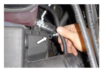
Release the clamp holding the MAF sensor wire from the corner of the airbox.
