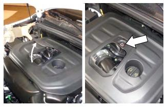
On the engine appearance cover, lift the access panel and remove. Then remove the screw and appearance cover.
