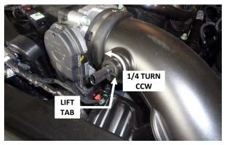
6. Remove the air temp sensor by lifting the locking tab and turning the sensor a quarter-turn counter-clockwise while pulling straight out. Store the sensor in a safe location until reinstallation.
