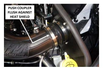
30. Push the flex coupler up against the heat shield and tighten only the filter adapter clamp.
