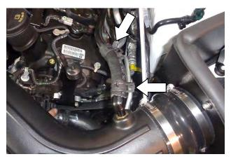
32. Push one end of the 5/8" I.D. hose (23) onto the PCV tube. Cut the hose to fit the barbed fitting in the intake tube, and secure at both ends using pinch clamps (22). NOTE: Point the ears on the clamps toward the heat shield, so that they do not hit the engine cover when it is installed at **Step 35**.
