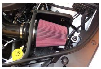
37. Place screw clamp (2) on air filter (1), install the filter on the filter adapter, and tighten the clamp.
