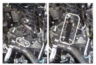
23. Locate the 2 screw holes on the engine as shown, and attach the bracket using M6 screws (8), lock washers (7) and flat washers (6).
