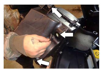
12. Remove any 2 of the 3 rubber mount grommets from the bottom of the airbox and retain for use at **Step 19**.
