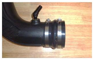
25. Install the 2 large screw clamps (18) on the 4" flex coupler (19). Then install the coupler on the filter end of the intake tube. **Do not tighten the clamps at this time.**
