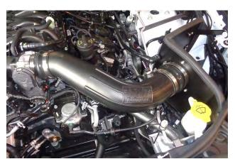
29. Install the intake tube in the vehicle, but do not tighten any screw clamps yet.
