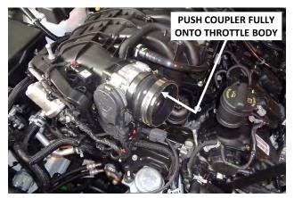
28. Install the medium and small screw clamps (25) and (27) on the 3-1/2" - to - 3" coupler (26). Push the coupler all the way onto the throttle body and tighten only the small (throttle body) clamp.
