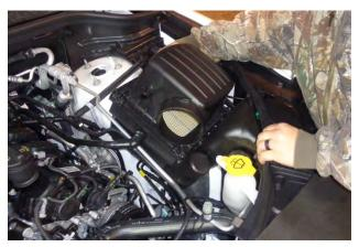
11. Remove the airbox from the vehicle by firmly pulling it straight up.
