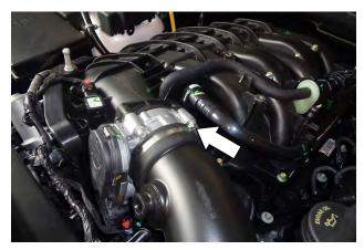
7. Loosen the screw clamp that secures the air inlet duct to the throttle body.
