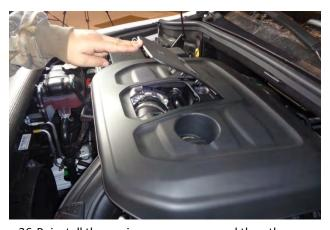
36. Reinstall the engine cover screw, and then the access panel.
