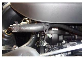
35. Verify there is no contact between the engine cover and the pinch clamp on the PCV tube. Adjust the pinch clamp if required.
