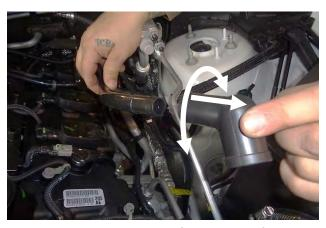
14. Remove the rubber elbow from the end of the PCV tube by carefully twisting it back and forth while pulling it straight off.
