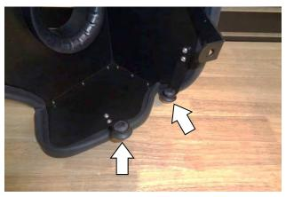
19. Push the two rubber grommets removed from the airbox at **Step 12** into brackets (12) and (11) as shown.
