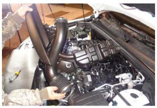
9. Separate the duct from the throttle body and the airbox, then remove it from the vehicle.
