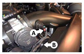
5. Disconnect the inlet air temperature sensor plug by lifting the latch (A) and pulling the plug straight off the sensor. Then carefully pry the wire loom clamp (B) from the resonator chamber.
