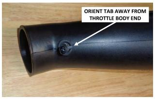
27. Carefully push the air temp sensor into the grommet, orienting the tab away from the throttle body opening. Moistening the grommet I.D. with soapy water will ease insertion. Note that the tab does not sit flush against the grommet – there will be a slight gap.
