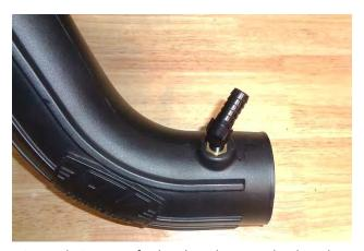
24. Apply 2 wraps of nylon thread tape to the threads of the barbed elbow (21), and install it in the intake tube (20).
