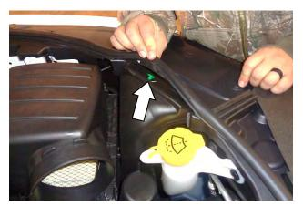
10. Lift enough of the engine compartment trim seal off the airbox snorkel to allow removal of the airbox.
