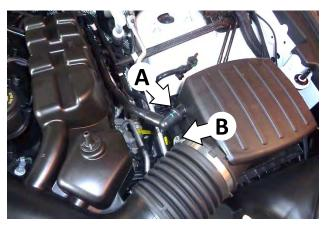
8. Disconnect the PCV hose from the airbox (A), then loosen the screw clamp (B) that secures the duct to the airbox.
