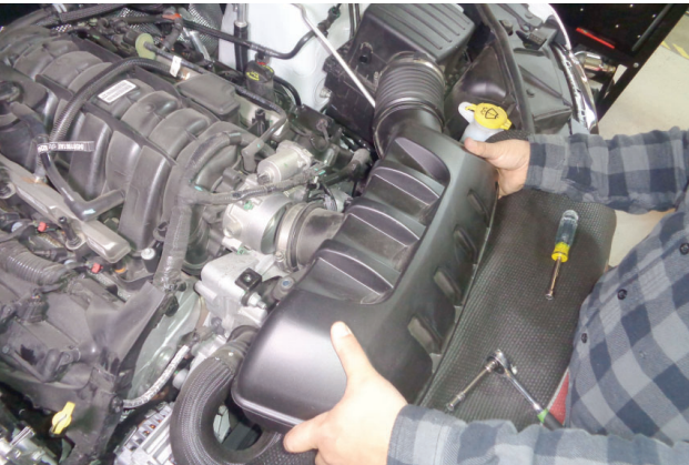
8. Remove resonator from engine compartment.
