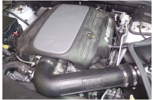
28. Re-install engine cover (removed step 3).
