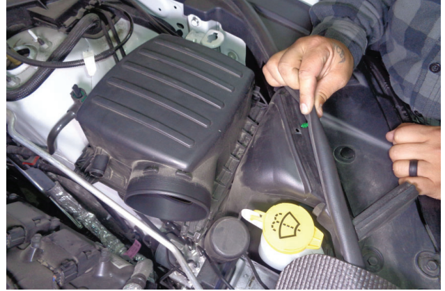
10. Unclip trim seal from corner of inlet duct.
