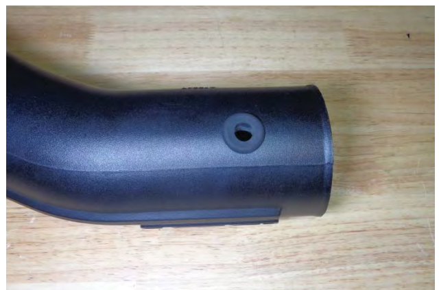
18. Insert the rubber grommet (22) into the intake tube (21). Moistening the grommet with soapy water will ease insertion.
