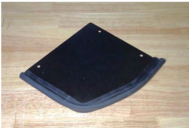
14. Attach gasket to the heat shield cover (5).
