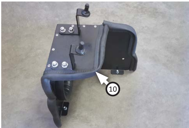
13. Wrap heat shield gasket (10) around edges of airbox, making sure it fits tightly. Once finished, keep remaining gasket for later use.
