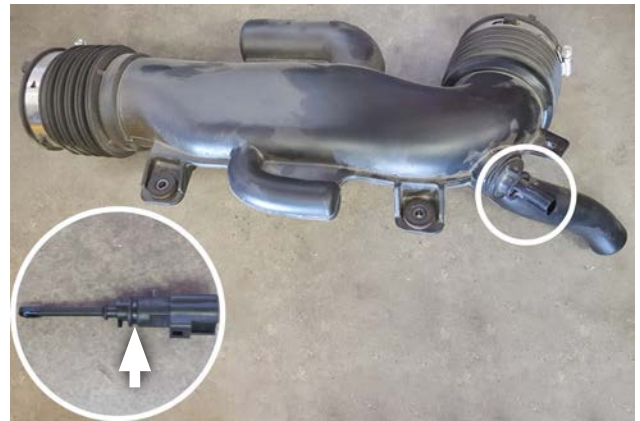
15. Remove IAT sensor from factory intake tube then remove o-ring from sensor.
