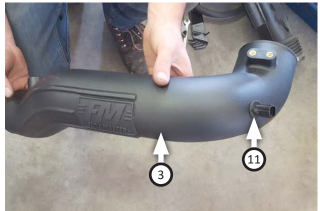
16. Fit grommet (11) into intake tube (3) then insert IAT sensor (from previous step) into it as shown.
