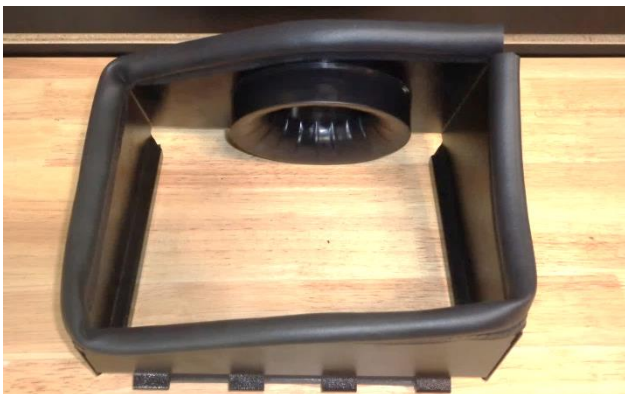
14. Firmly press the gasket (5) onto the edge of the heat shield, gradually working your way around. When you return to the starting point, use metal-cutting shears to trim the gasket to length.
