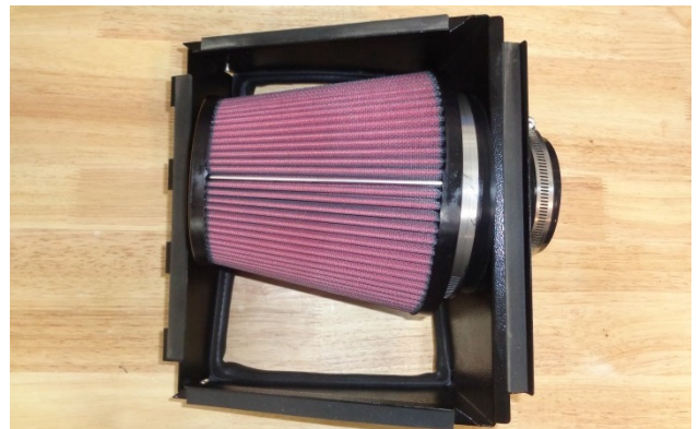
17. Slip screw clamp (2) onto the air filter (1), then install the filter on the filter adapter and tighten the clamp.
