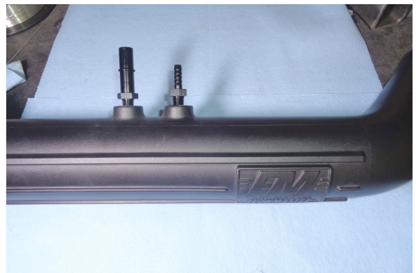
18. Your vehicle may require either the 5/8" quick connect (QC) fitting (16), or the 3/8" barbed fitting (17), or both. If it uses only one fitting, install the 1/4" plug (20) in the unused port. Apply 2 wraps of nylon thread tape to threads of the required hardware, and install them in the intake tube (12).
