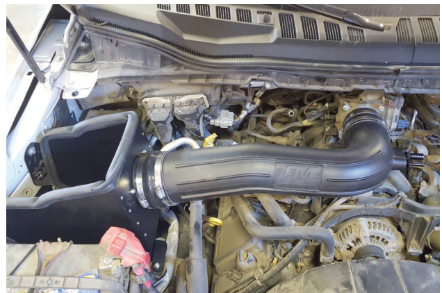
17. Place intake assembly into engine compartment between airbox and throttle body. Press couplers against stops then center tube. Tighten screw clamps completely.
