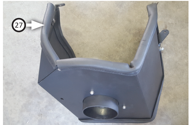
15. Wrap airbox trim seal (27) around edges of airbox and bracket 2, making sure that it fits tightly then trimming any extra if necessary.
