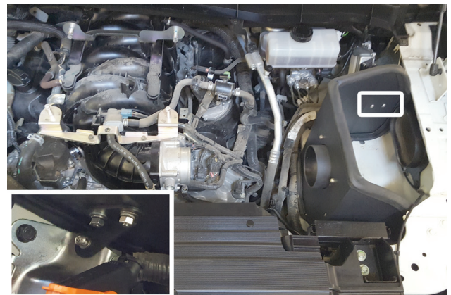
17. Fasten airbox to vehicle frame using bolt (14) , flat washer (12) and split lock washer (13) through bracket 1.
