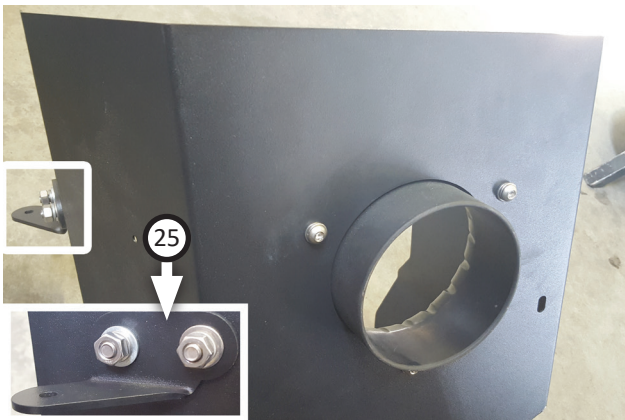
13. Install bracket 2 (25) onto airbox using (x2 ea.) bolts (26) , flat washers (5) , split lock washers (6) and nuts (7) .
