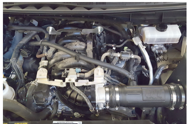
28. Inspect all connections, making sure they are firm and properly seated. Make sure intake tube is centered and that its logo is facing upward.
