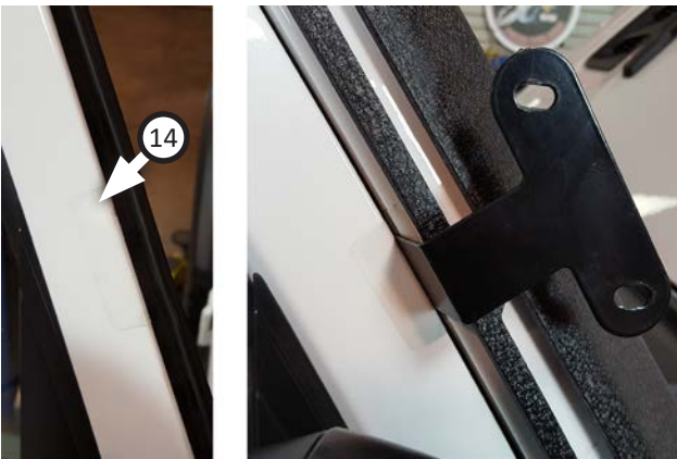
25. Carefully close passenger door, align door gasket (14) on outside so it protects door from rubbing against bracket 3 then apply it to front/inside.
