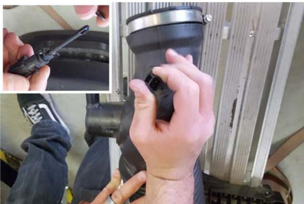
**Note orientation of air temp sensor for reinstallation.**
