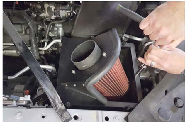
11. Install the heat shield and filter assembly on the airbox with 5 stock screws.
