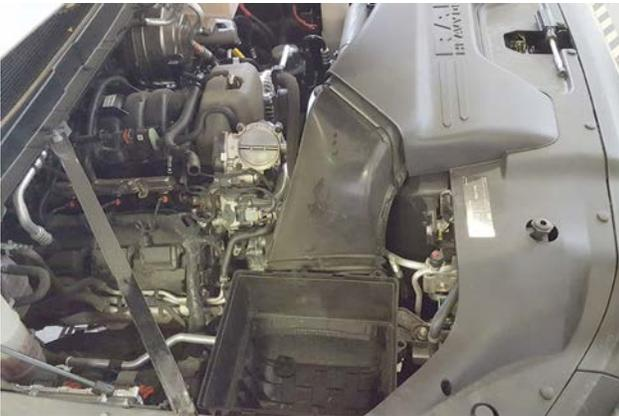
7. Remove the air filter from the factory airbox.
