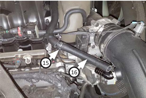
19. Place **pinch clamp (15)** over **hose (16)**, then push the hose onto the stock PCV hose fitting. Move the pinch clamp over the fitting to secure the hose.
