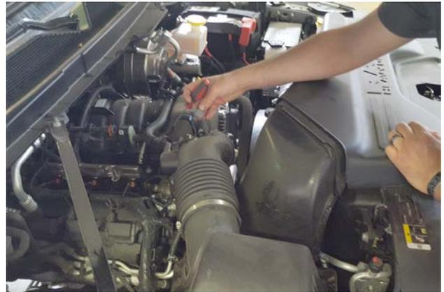
3. Disconnect the air temp sensor lead from the sensor.
