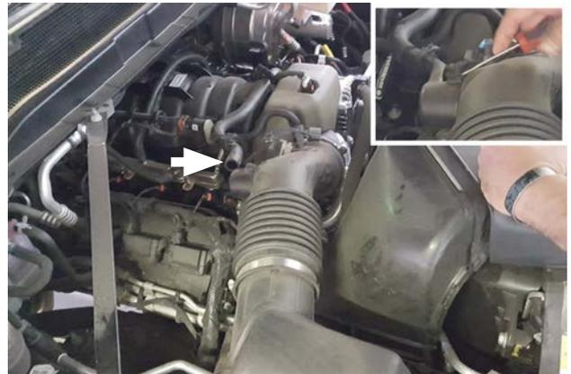
4. Remove the PCV hose from the intake tube, and remove the wire holder from its end.
