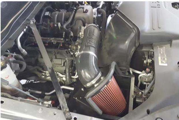
14. Install the intake tube assembly. First, push the reducer coupler fully against throttle body stops and tighten the clamp. Then push the elbow coupler up against the heat shield. Finally, center the tube between the couplers with the logo facing up, and tighten the remaining clamps.
