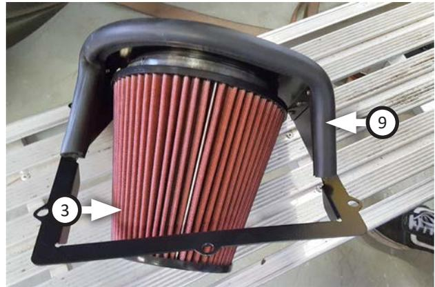
10. Push **gasket (9)** onto the edge of the heat shield as shown, cutting off the excess length with metal shears. Install the **air filter (3)** onto the adapter with the included clamp.
