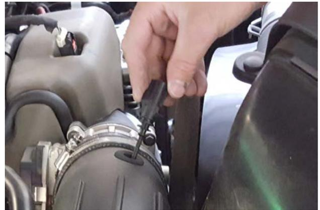
15. Install the air temp sensor into the grommet in the intake tube. Orient the sensor as noted at removal.
