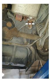
5. Remove fasteners from inlet pipes then disconnect and remove muffler sections from vehicle.
