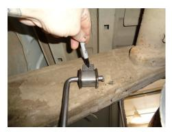
6) Adjust the exit pipe so that the tips are the desired distance from the body, then rotate the **HA572** hanger so that it lays flat against the inside of the vehicle frame and use a center punch to mark the center of the two holes on the frame. Rotate the hanger out of the way and drill each mark using a ¼" drill bit. Use the two 5/16" thread cutting bolts to secure the hanger to the frame. Tighten securely.
