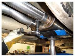
Place a supplied 2-1/2" clamp onto each muffler outlet. Place the exit pipe assembly **#86465M** up into position and slide into both muffler outlets approximately 2". Use a stand to support the outer end of the assembly. Tighten the clamps just enough to hold in position.
