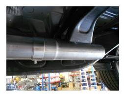
2) If installing the system on a Crew Cab truck with a 6.5' bed, place extension pipe **#TB700M** onto the back of the **#26687M** inlet pipe, place a provided clamp onto the slip-fit and tighten enough to hold in position. This extension pipe will not be used on Double Cab or Crew Cab-5.5' bed models.
