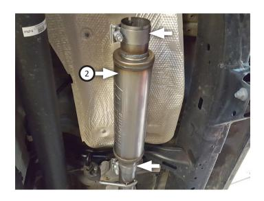
10. Route overaxle assembly (3) over axle and connect it to muffler then insert wire hangers in mounts. Place clamp (5) onto exit pipe assembly (4) and connect it to overaxle pipe. Tighten clamps enough for adjustment.
