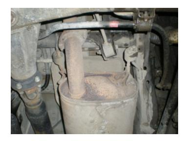
4. Remove (x2) factory spring loaded bolts at inlet pipe flange connection and set aside. Retain bolts and springs for later use.
