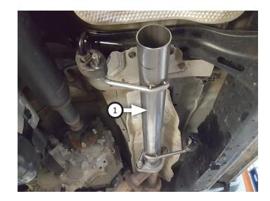
9. Place (x2) clamps (5) onto FFX muffler (2) then connect it to inlet pipe. Tighten front clamp just enough to allow for adjustment.
