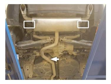
4. Remove muffler assembly from vehicle then transfer isolator mounts over to FFX muffler.
