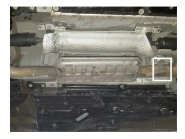
www.flowmastermufflers.com Technical Support (866) 464-6553  Place clamp (6) onto front inlet pipe (1) then connect it to factory pipe, lining inlet pipe notch up to factory pipe tab as shown below. Place clamp (6) onto mid pipe (3) and connect it to front inlet pipe. Tighten clamps just enough to allow for later adjustment.
