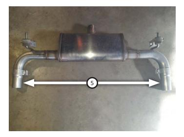
12. Place **clamp (6)** onto muffler assembly then connect it to tailpipe. Re-bolt hanger mounts, then tighten clamp just enough to hold parts.
