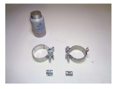
6. Place clamps (x2) (3) onto left (1) and right (2) mufflers then connect them to exhaust and insert wire hangers (x2) into isolators. Secure muffler ends with nuts and muffler/pipe hangers (removed step 4).
