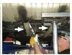
4. Dismount both front wire hangers, remove nuts (x4) and muffler/pipe hangers (x2) from muffler rear then disassemble and set aside muffler from vehicle. Retain nuts and muffler/pipe hangers for later use.
