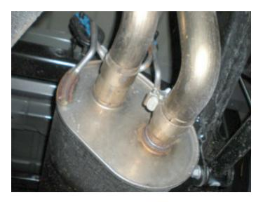
Loosen clamp on muffler inlet, then remove hangers (x2) at muffler rear from isolators. Slide muffler rearward to disconnect it from inlet pipe then lower and set it aside.
