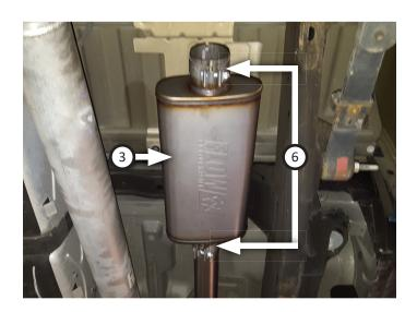
9. Route **tailpipe assembly (4)** over axle and connect it to muffler outlet. Mount wire hangers into isolators (x3) then tighten clamp enough to allow for adjustment.
