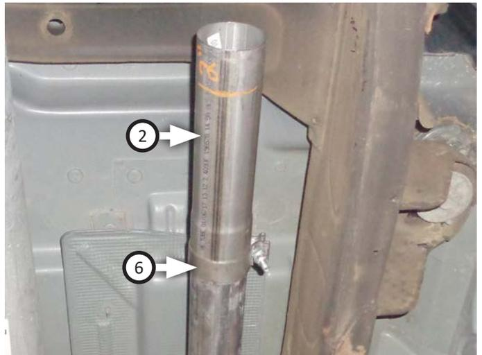
10. Place **clamp (6)** onto **muffler (3)** then connect it to inlet/extension pipe. Tighten clamp just enough to allow for adjustment then place **clamp (6)** onto muffler outlet.
